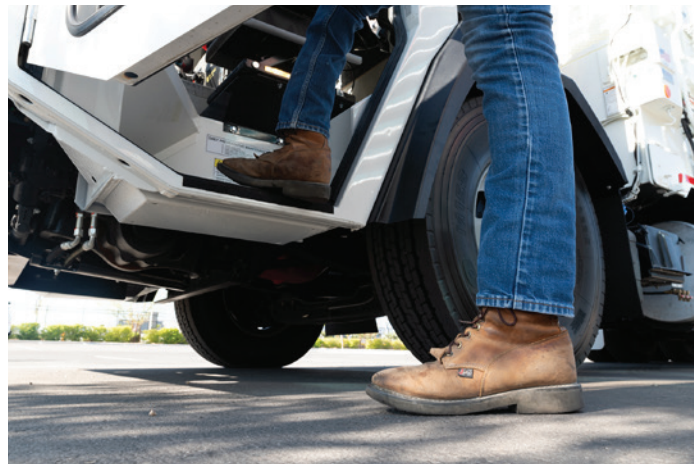
True low entry 18" step-in height on both sides
