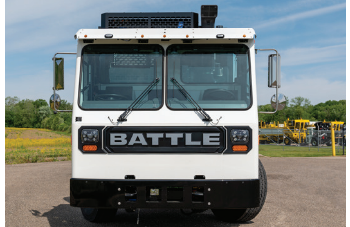
82" cab width engineered to be 12" narrower than our standard chassis for tight applications
